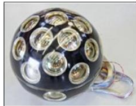
Each Digital Optical Module (DOM) is a standalone sensor module with 31 3-inch PMTs in a 17-inch glass sphere.
